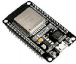
Gambar 2. 1 Modul ESP32
